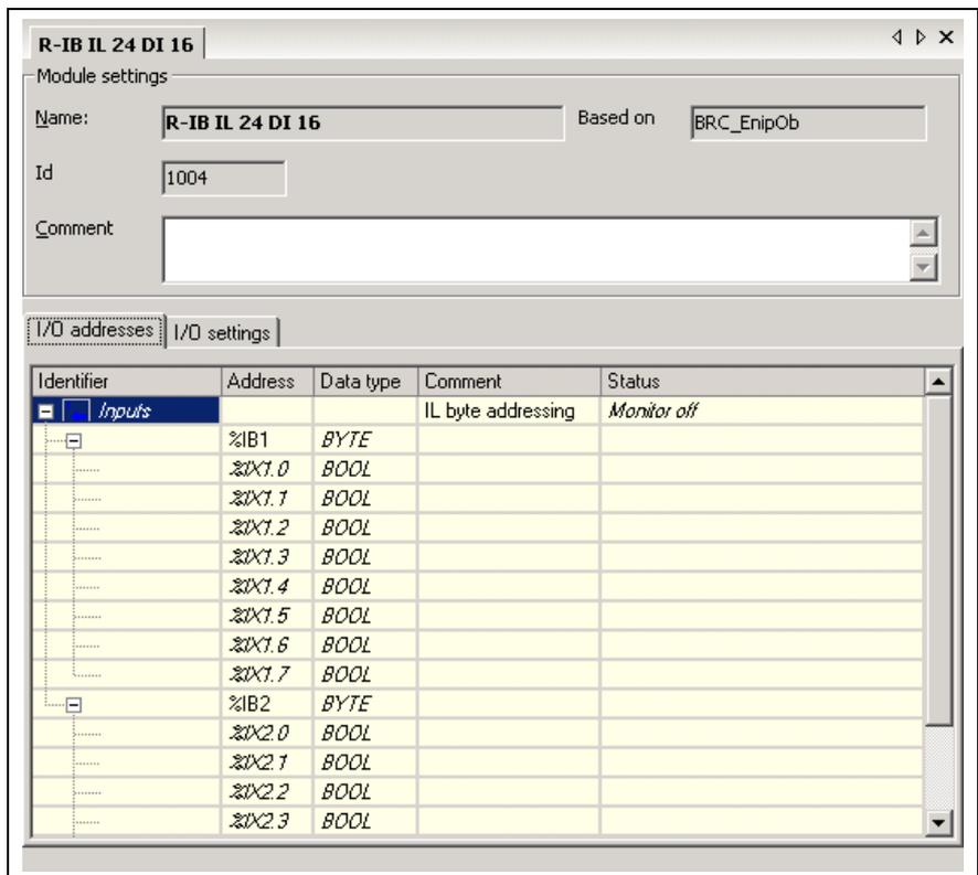
Fig. 4-21: Window of an Inline module (example)
