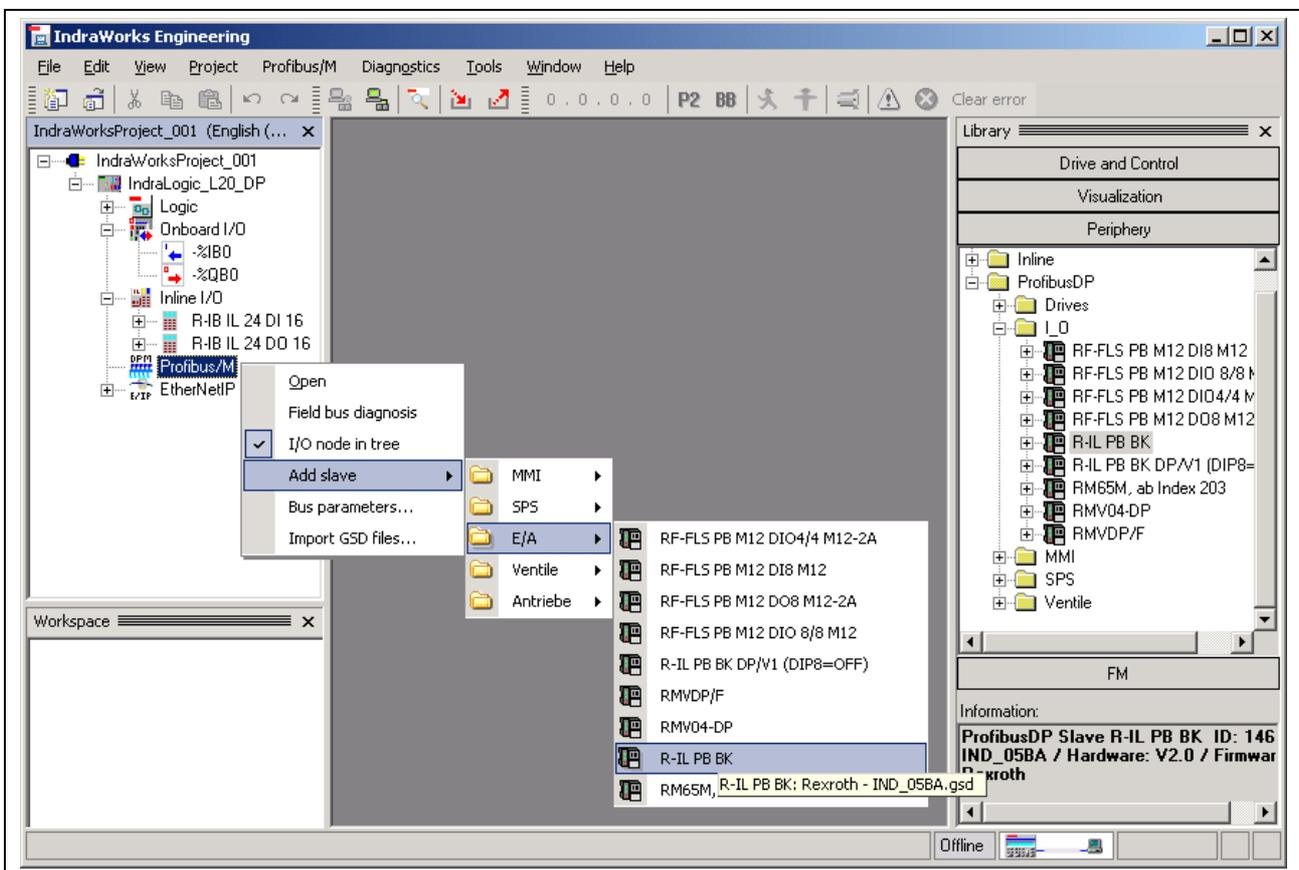
Fig. 4-25: Inserting a Profibus DP slave via the context menu of the "Profibus/M" object
