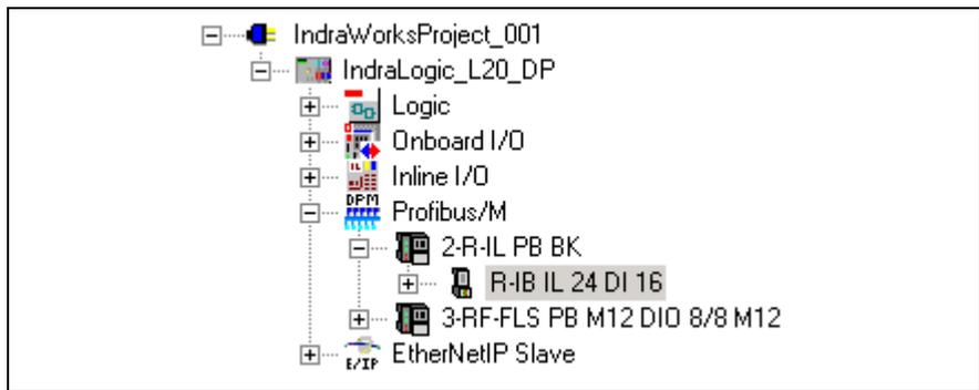
Fig. 4-33: Module of a Profibus DP slave (example)
