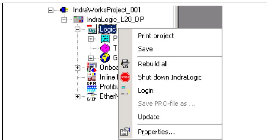
Fig. 5-3: Context menu of the "Logic" object when the IndraLogic is **started**
