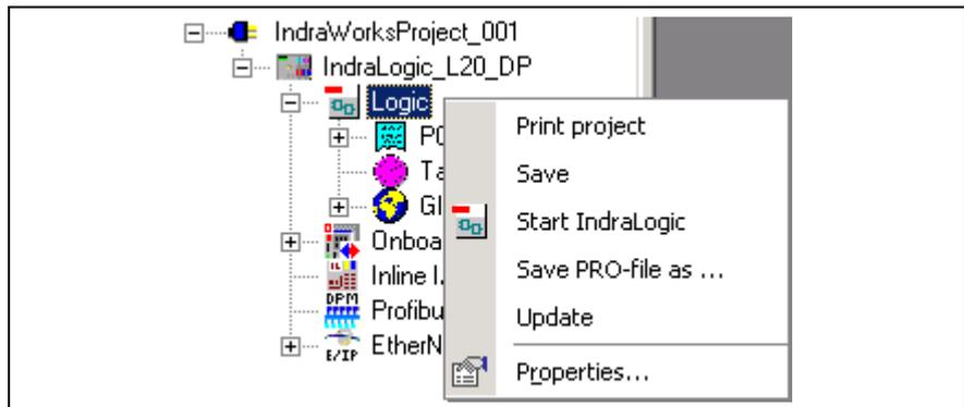
Fig. 5-4: Context menu of the "Logic" object when the IndraLogic is **not started**
