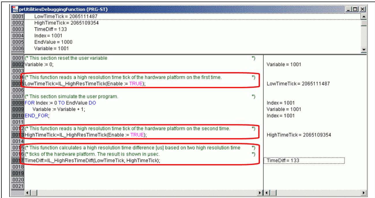
Fig. 6-95: Application example of the IL\_HighResTimeTick function
