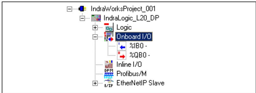
Fig. 4-15: "Onboard I/O" object
