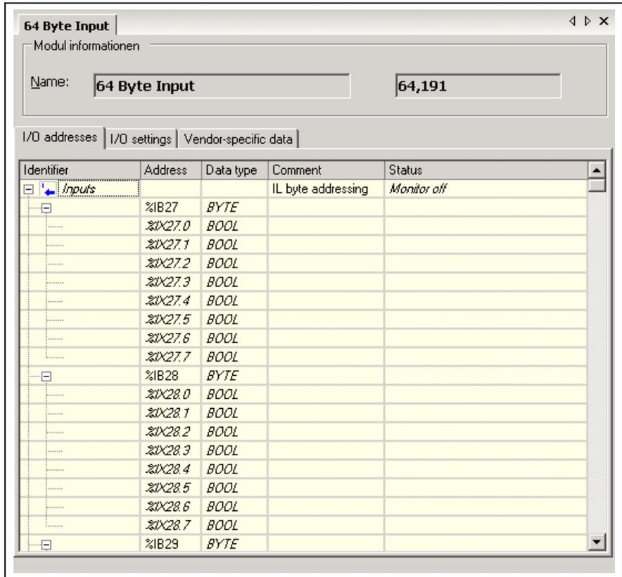
Fig. 4-38: Coupling area of a "Profibus/S" object (example)
