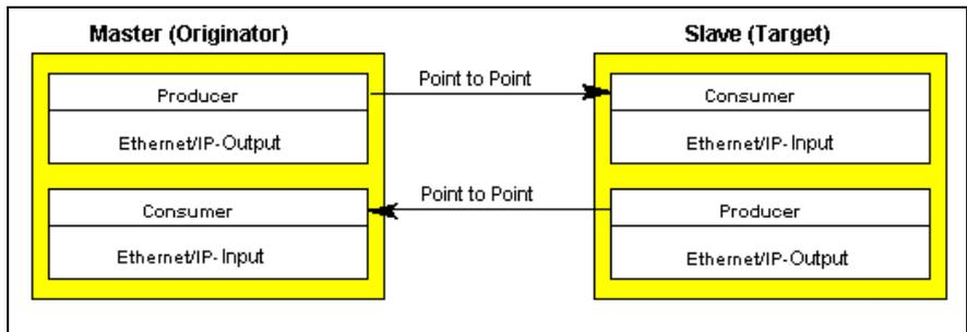
Fig. 4-45: Ethernet/IP connection type: Point to point
