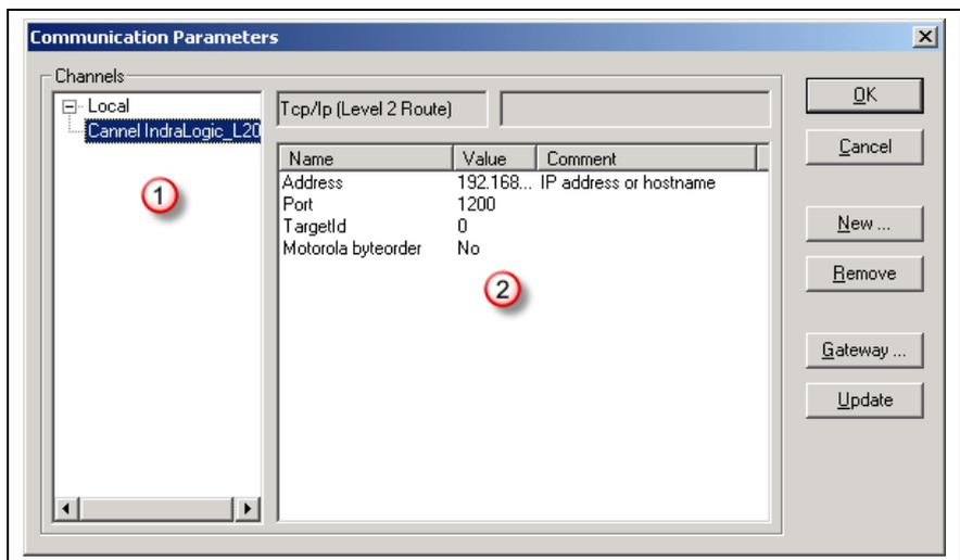
Fig. 4-8: Adapt the parameters of a communication channel
