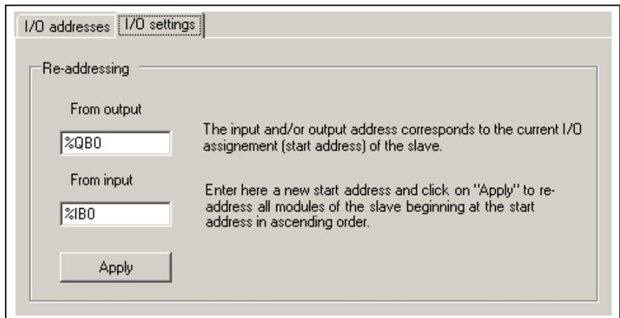
Fig. 4-18: Readdressing the onboard I/O
