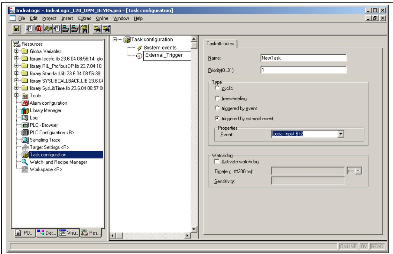
Fig. 4-54: IndraLogic task configuration
