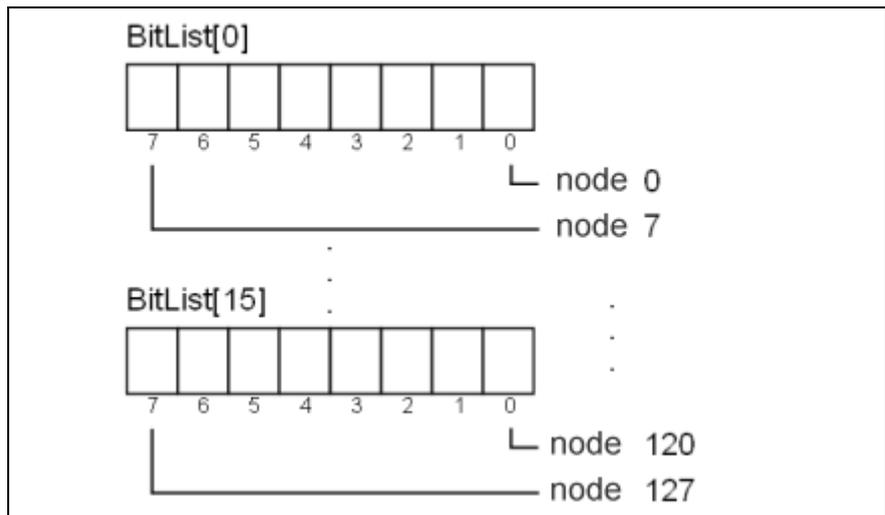
Fig. 6-45: Coding of the bit list
