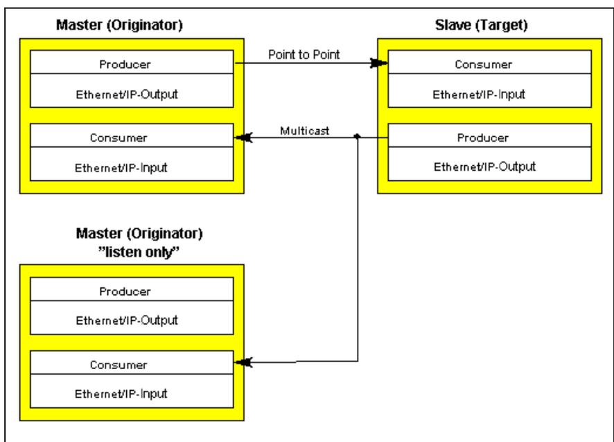
Fig. 4-46: Ethernet/IP connection type: Point to point / multicast
