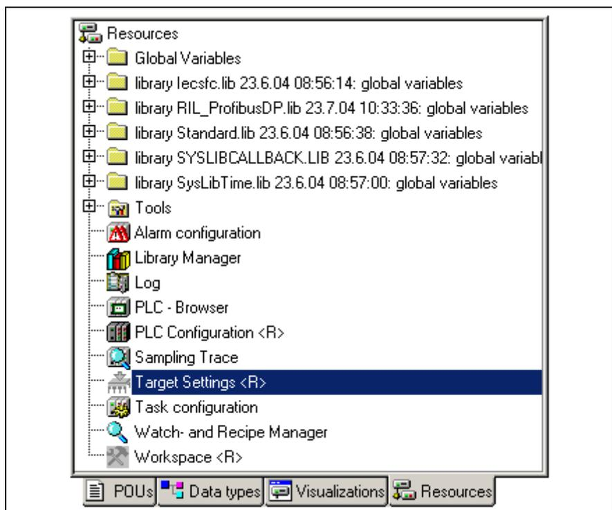
Fig. 4-52: IndraLogic, resources, "target settings" object
