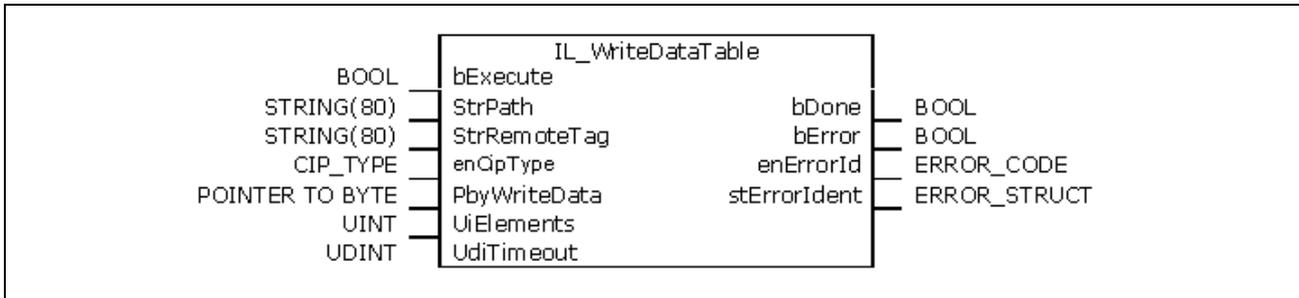
Fig. 6-28: Structure of IL\_WriteDataTable
