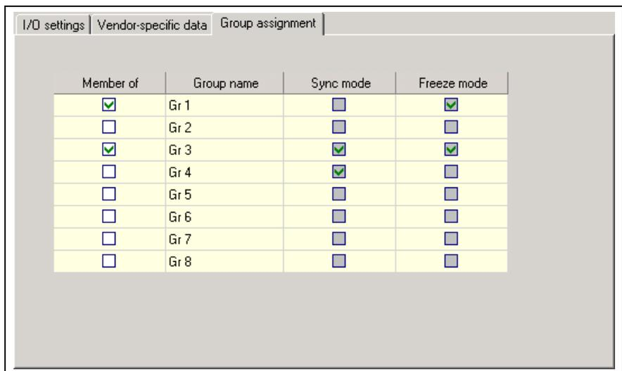
Fig. 4-31: Group assignment of a Profibus DP slave (example)
