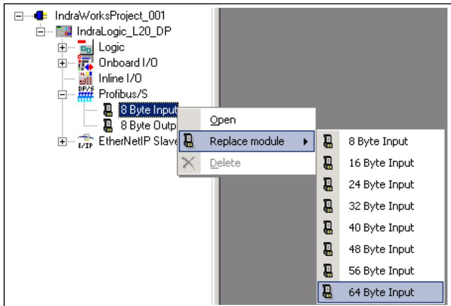
Fig. 4-37: Select data capacity for input/output area
