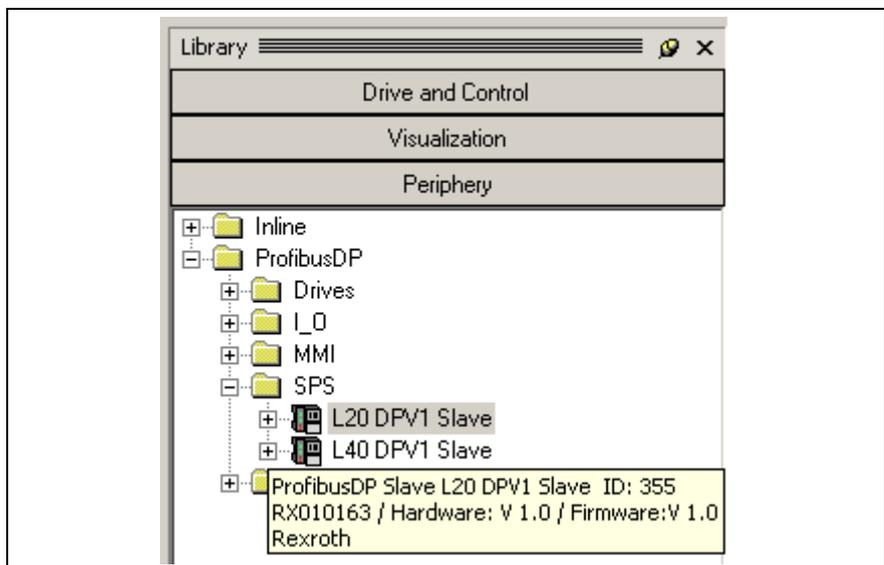
Fig. 4-39: Projecting the IndraLogic L20 in the superordinated control as slave (device in the library)
