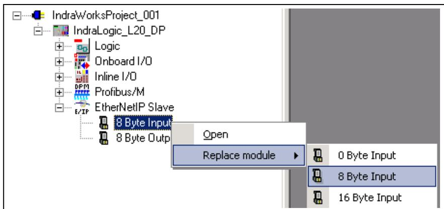
Fig. 4-43: Select the data capacity for the input and output box of the Ethernet/IP slave
