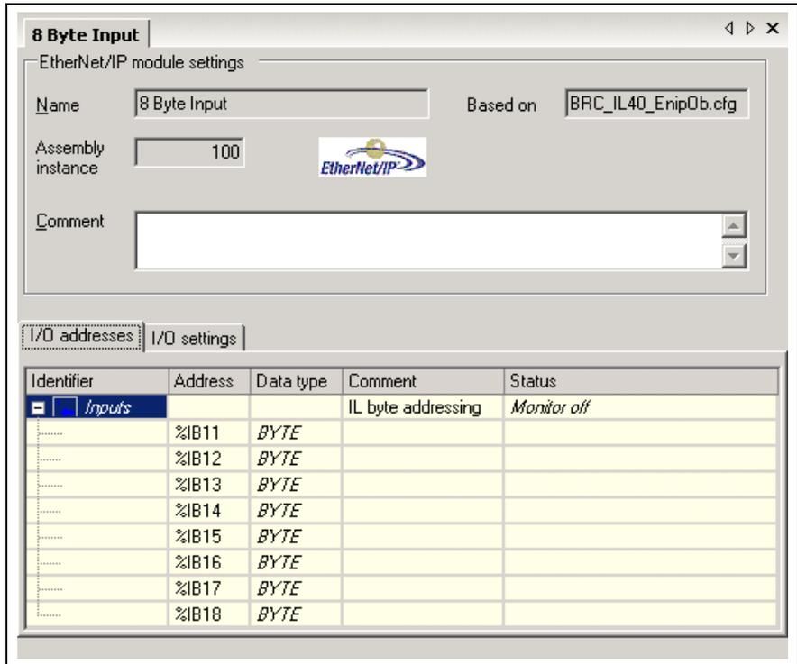
Fig. 4-44: Coupling area of an "Ethernet/IP slave" object (example)
