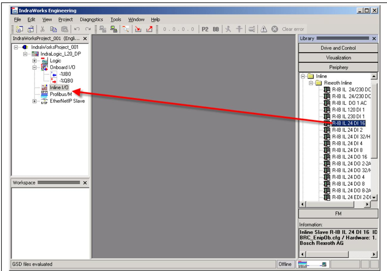
Fig. 4-19: Insert Inline module (example)
