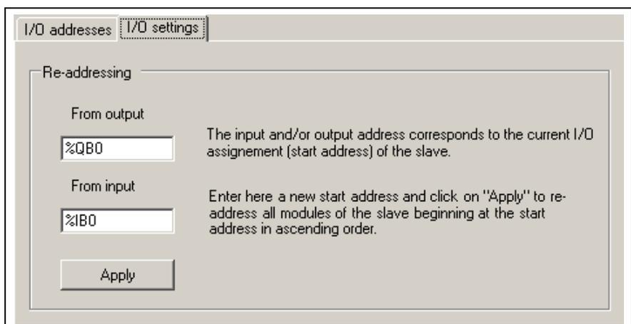
Fig. 4-22: Readdressing an Inline module
