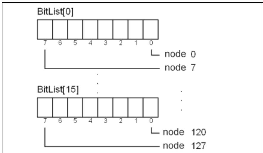
Fig. 6-48: Coding of the bit list
