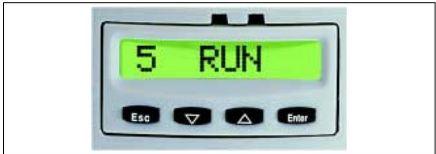
Fig. 7-1: Display with operating keys
