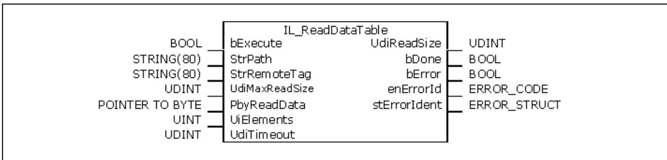
Fig. 6-24: Structure of IL\_ReadDataTable
