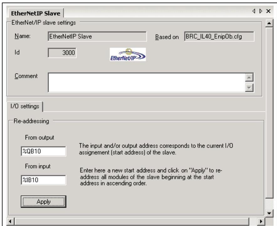
Fig. 4-42: "Ethernet/IP slave" window
