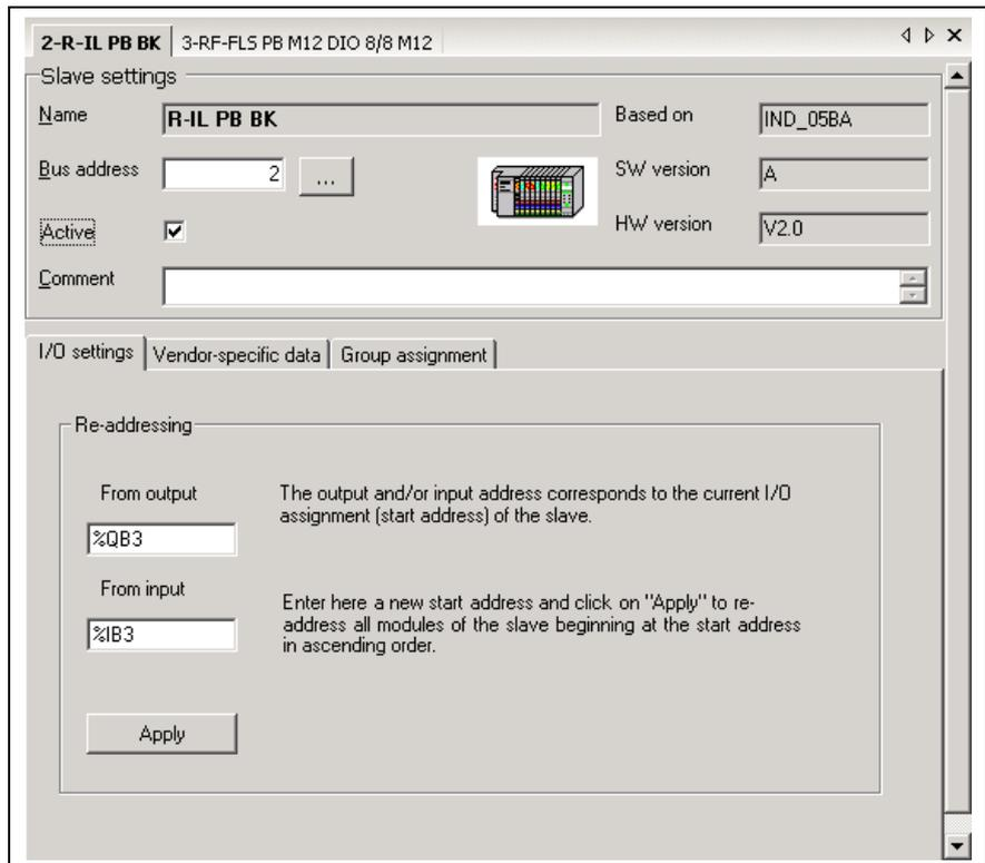
Fig. 4-27: Window of Profibus DP slave (example)
